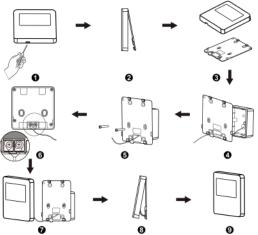
Fig. 4.10 Installation of Wired Controller
