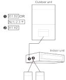
Fig. 4.5 two wired controllers control one indoor unit
