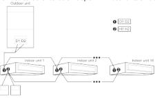
Fig. 4.7 two wired controllers control multiple VRF indoor units simultaneously
